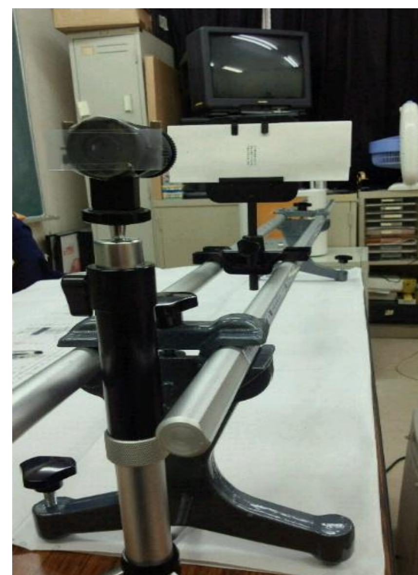
Figure 3. Target letters are set on the optical bench
