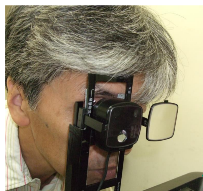
Auto-focus telescope with attachment lens of 3D and 6D
